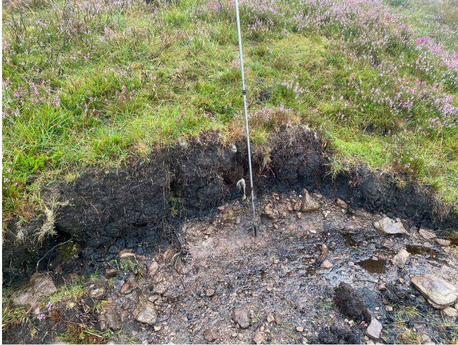
Plate 8-2 Typical profile - peaty topsoil layer over gravelly glacial till (Knocknanask)
